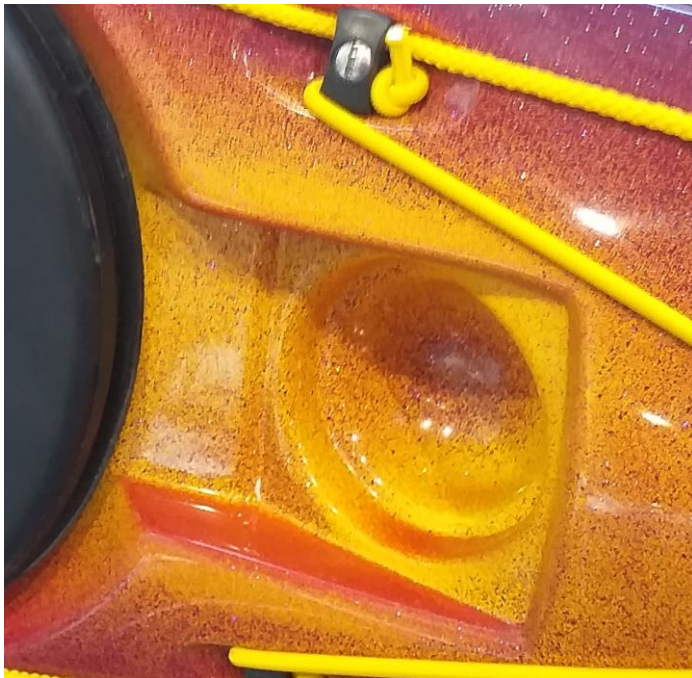
Faded gel coat, stripes, different densities and colour of glitter.
