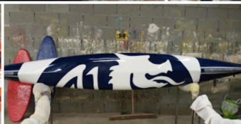
Faded gel coat, stripes, different densities and colour of glitter.
